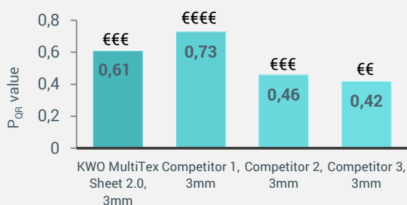
Fig. 1: Creep/relaxation test acc. to EN 13555 (stiffness 500 kn/mm, initial sealing performance 30 MPa, 150 °C, DN40/PN40)
