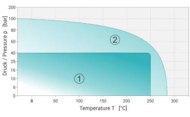
The p-T diagram indicates the service limits considering the simultaneous influence of pressure and temperature.
