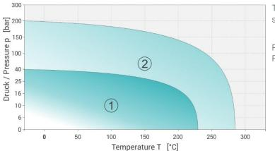
The p-T diagram indicates the service limits considering the simultaneous influence of pressure and temperature.
