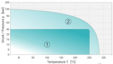
The p-T diagram indicates the service limits considering the simultaneous influence of pressure and temperature.
